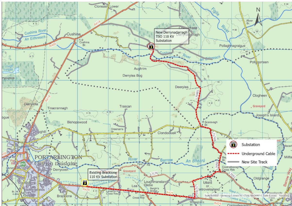
Figure 1.1 – Grid Connection Route
